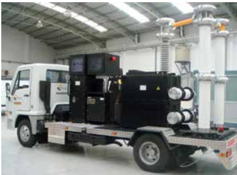
200kV VLF Withstand, VLF TD & VLF PD Test Truck Inducor Ingenieria S.A. Argentina
