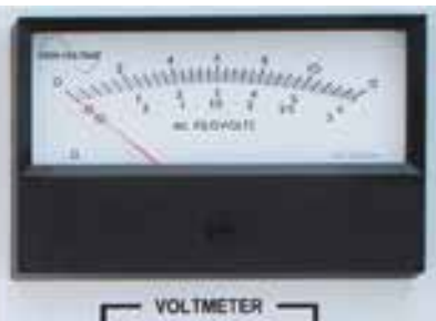
Two ranges for each output voltage tap 6 kVac Output: 0 - 3 kVac & 0 - 6 kVac 12 kVac Output: 0 - 6 kVac & 0 - 12 kVac
