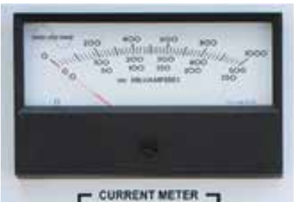
Three ranges for each output voltage tap 0 - 250 mAac, 0 - 500 mAac, 0 - 1000 mAac
