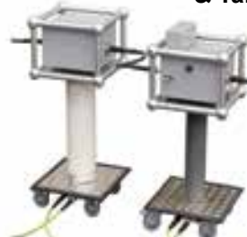
Shown is PDIX-70, 70 kV peak models to 200 kV available
